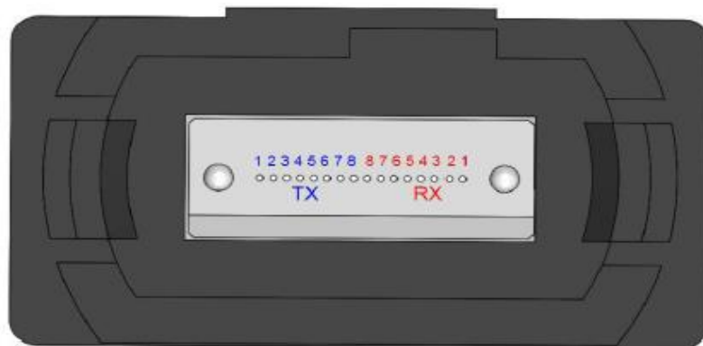
Figure 3. MPO-16 Optical Connector Interface
